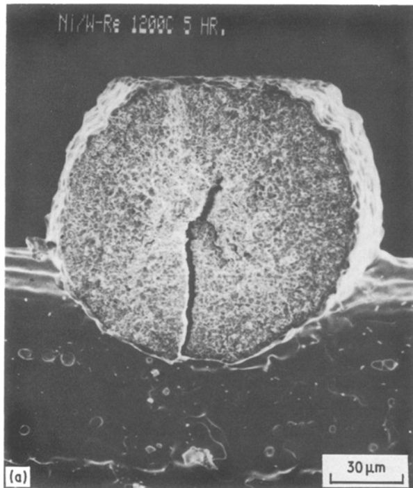
Figure 7 Fracture surface of Ni/W–Re wire exposed to 1200° C for 5 h.
